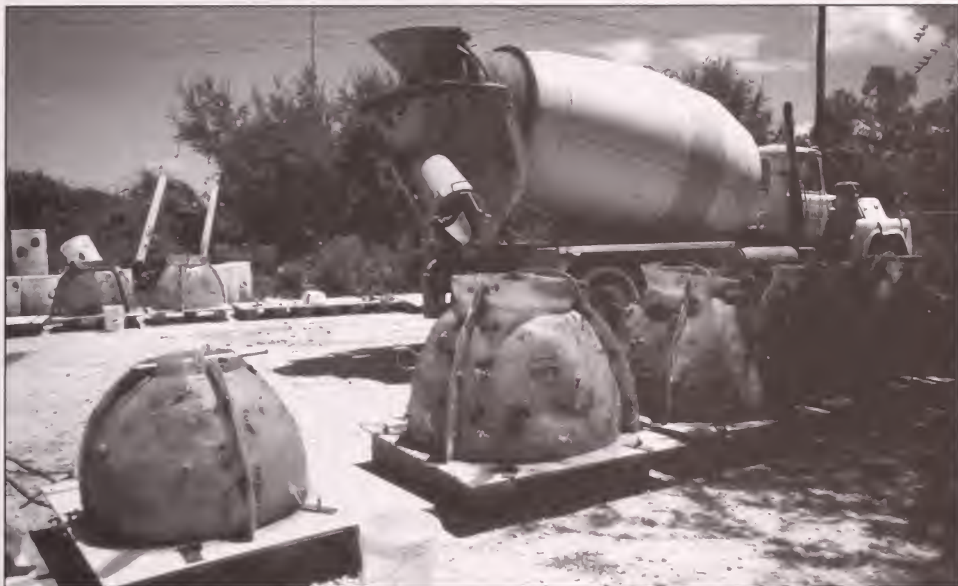
Eternal Reefs mix cement and cremated remains to rebuild habitats for sea life.
