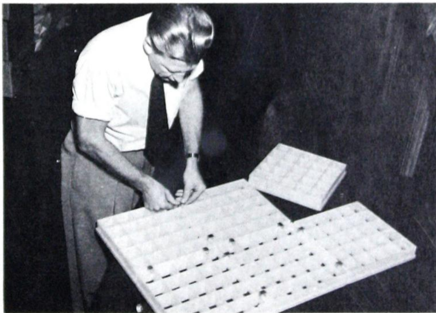
CLIPPING "LUVE-TILE" MODULAR SQUARES TOGETHER FOR DOORS. LAY ON LEVEL SURFACE AND PRESS CLIPS ON WITH THUMB
