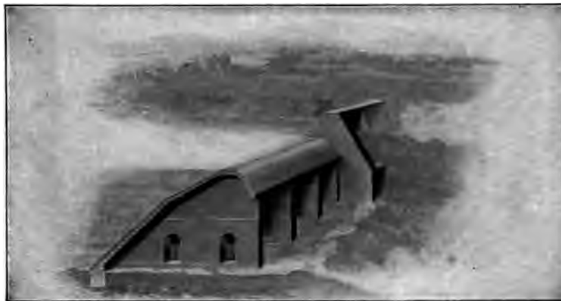
FIG. 43.—SECTION OF CONCRETE-STEEL CURTAIN-DAM.
