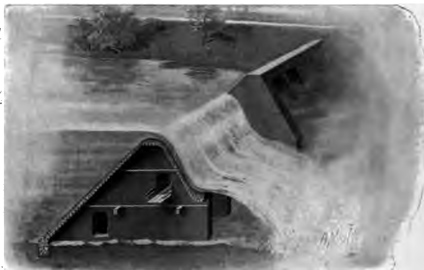
FIG. 45.—SECTION OF CONCRETE-STEEL HALF-APRON DAM FOR ROCK FOUNDATION AND HIGH HEAD.
